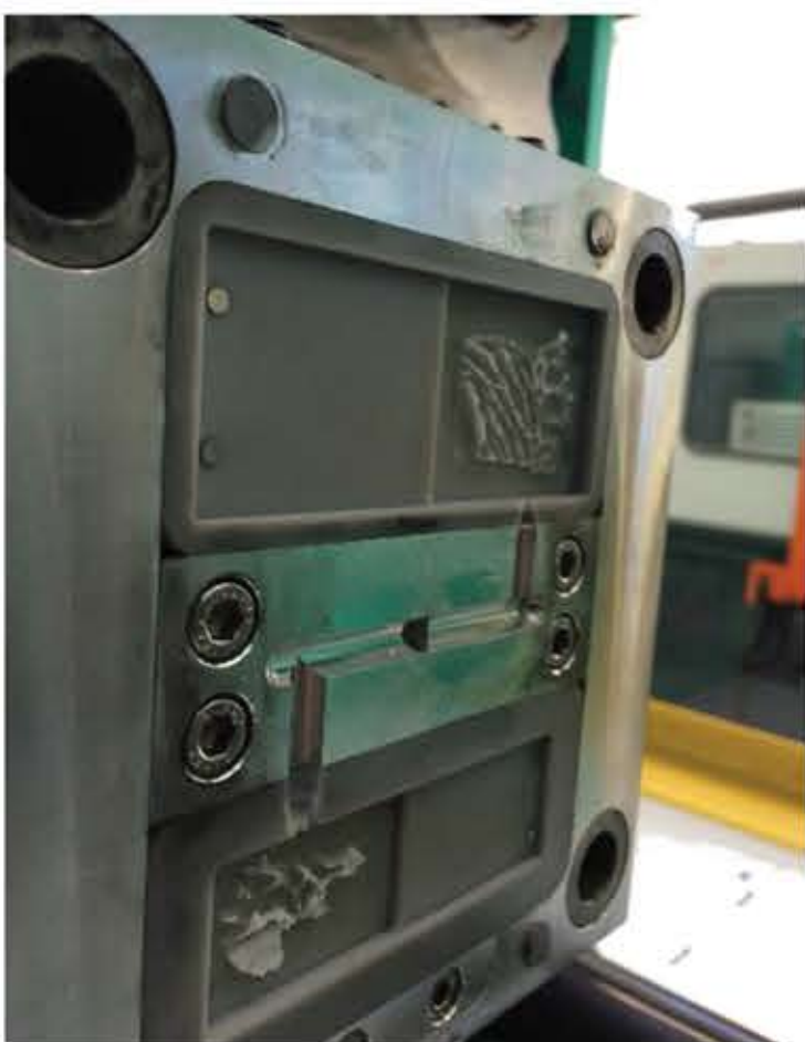
Figure 1 – Simple block cavity with mould deformation
